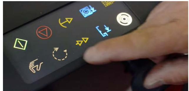
The inputs and outputs are managed by **EtherCAT** bus systems. Thanks to an EtherCAT-ASi gateway realized in CODESYS, the program manages the communication with about one hundred I/O points on the machine such as the ASi pushbuttons present onboard the machine near each printing cylinder that allows their manual management.
