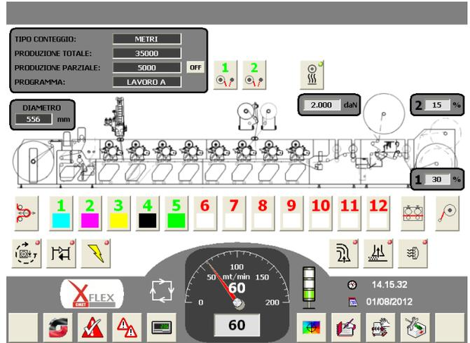
In addition to the Premium HMI functionalities and thanks to the flexibility of the tools provided by the Windows platforms, OMET has added internally developed programs for **data exchange between machines of the same plant for the synchronization of information related to production recipes**. The same application also supports the creation of **reports** for production monitoring.
