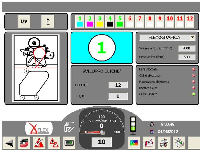
The HMI application implements the classic controls that allow the display of the machine **status**, the display of **alarms**, the consultation of the history of **events** that occurred, the management of the various **formats**, settings, and parameterizations. Particularly interesting for the type of application is the management of the various types of formats through Premium HMI’s powerful data archiving tools that use databases for reliable archiving even of considerable amounts of data.
