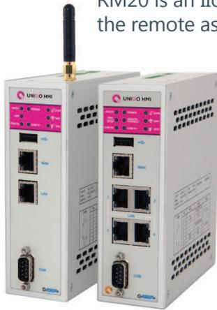
RM20 is an IIoT gateway that combines the remote assistance functionalities of the UBIQUITY platform with the programming potential of UNIQO making it an ideal system for the realization of IIoT gateway solutions. Thanks to the integration of UNIQO software is possible in fact to create an intelligent and totally dynamic application that can perform all the required operations.
